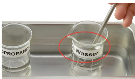
Fig. 2 Sensing head in deionized water
